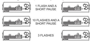
Press the vehicle remote control lock/unlock buttons to make sure the alarm system works properly. Eventually disconnect the 8-pin connector and reconnect it after a few seconds.
